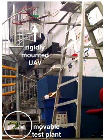
Fig. 6: Setup of tests used for characterizing downwash. The sUAS was attached to a ladder, and a plant (bottom left) was manually moved around beneath the robot. We visually observed leaf perturbation from downwash.
