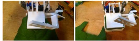
(a) Image of our final iteration holding a leaf. (b) The leaf after cutting operation.
