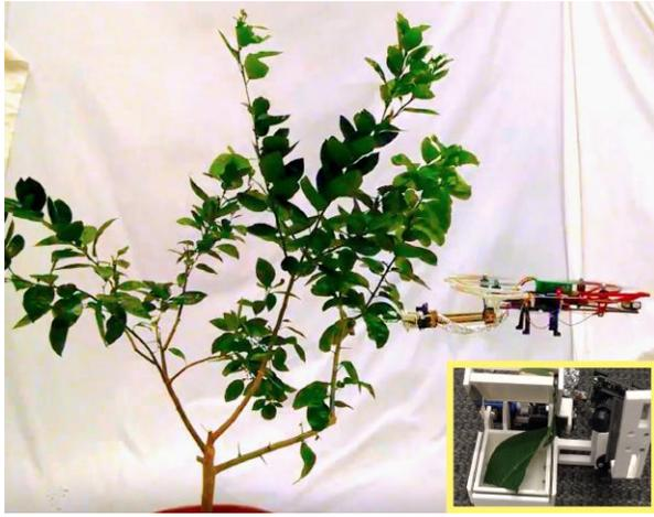
Fig. 2: The system during a flight trial, severing and storing a citrus leaf. Inlay at bottom-right shows the gripper mechanism with the acquired leaf sample. The storage box lid prevents contamination during specimen transport.
