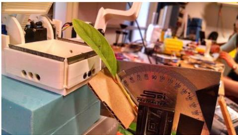
Fig. 10: Setup of angle variation test experiment. Boxes were used to vary the height of the gripper so that the leaf could be grasped at the angle measured with the protractor.
