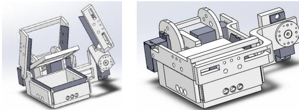
(a) Final iteration in open configuration. (b) Final iteration in closed configuration.
