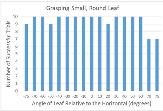
Fig. 9: Ability to grasp small, round leaf over 10 trials. The shape of this chart is representative of the other angle measurement tests performed.
