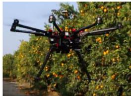
Fig. 1: This work addresses phytobiopsy using UAVs that fly close to symptomatic trees and acquire leaves autonomously for ex-situ analysis.
