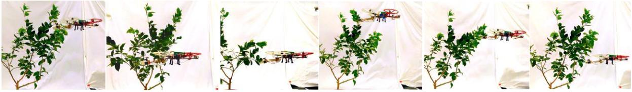
Fig. 14: Images showing contact during 6 successful manual indoor flight trials on the citrus tree, in different configurations. Note that the effect of downwash is absent, due to the extended arm design.
