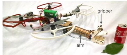
Fig. 4: The phytobiopsy UAV, with the gripper and the arm assemblies highlighted. The soda can is for scale.
