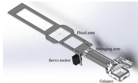
Fig. 5: CAD model of extendable arm, showing the servo motor for extending and retracting the arm.
