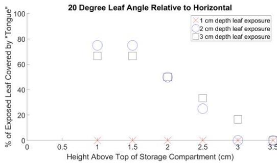
Fig. 12: Results of depth test with a paper leaf sample (for repeatability). The y-axis is normalized based on the depth of emulated leaf exposure. The linear trend shows that the ability to grasp leaf samples drops off as they move farther away from the storage box along the gripper’s vertical axis.
