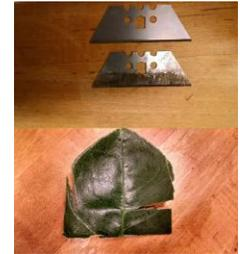
Fig. 17: Top: The new blade compared to the blade with plant matter build-up. Bottom: The partial cut was from an attempt with the old blades; the complete cut was from an attempt with the new blades.
